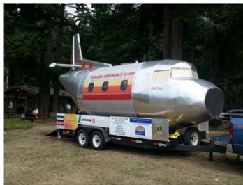
Part Embraer airliner fuselage with a custom built DC 3 looking nose and Hercules tail sections, the AirBuzz Mk II provides a great platform for a realistic flight simulator. The "X-Plane" FS program is both challenging and realistic. Students can make simulated flights to anywhere on the planet.
