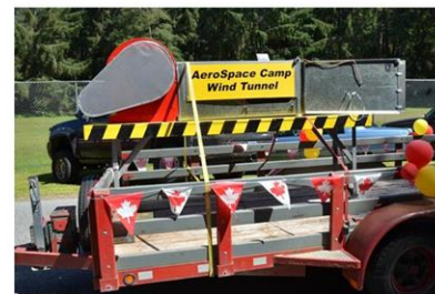
The wind tunnel is computer controlled. It measures drag, speed, vibration and lift of airfoils. A specially mounted model airplane can be flown remotely in the tunnel
